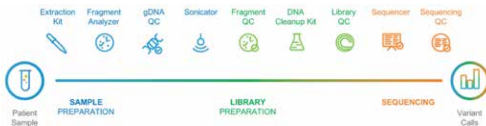
Figure 1: Overview of the NGS Workflow. The workflow can take up to 3 days to complete and involves many steps.
