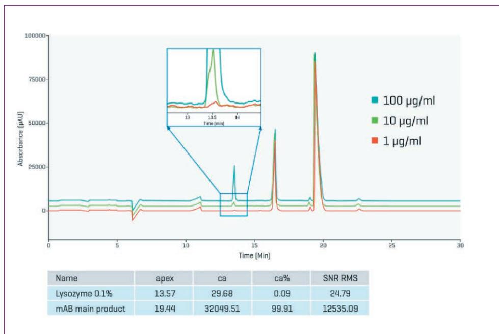
**Figure 4:** Sensitive Quantitation. Regulators commonly require quantitation down to 0.1% for impurities. The BioPhase 8800 system with UV detection detects 0.1% lysozyme spiked into 1000 µg/ml of IgG.
