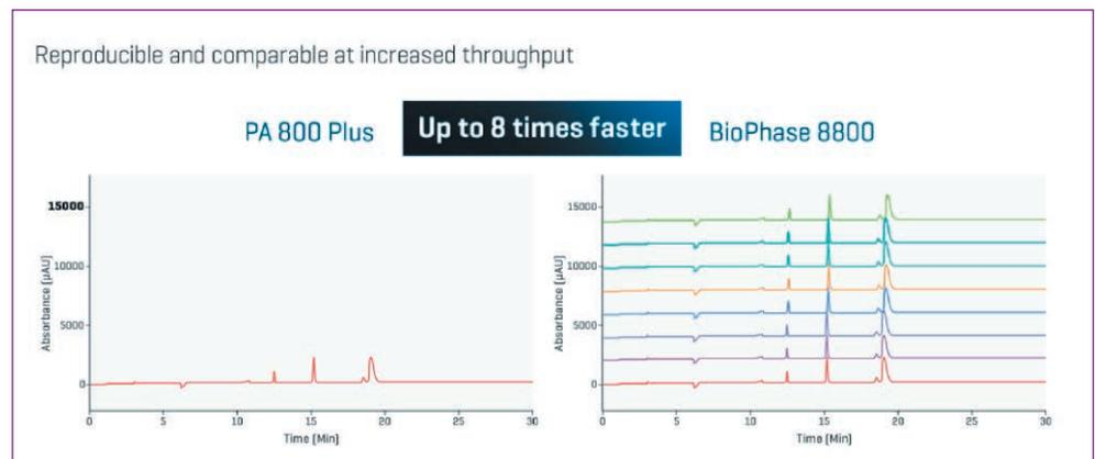
**Figure 2:** Processes Eight Samples in Parallel. Comparative of SDS-CGE separations of the reduced mAb sample on the multi-capillary BioPhase 8800 system and the single capillary PA 800 Plus Pharmaceutical Analysis system.
