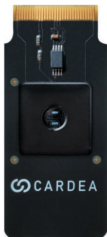
Figure 3: A standard Cardean chip containing multiple sensors inside the circular well.
